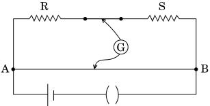
In a meter bridge shown in the figure, the balance point is found to be 40 cm from end A. If a resistance of 10  $\Omega$  is connected in series with R, balance point is obtained 60 cm from A. Calculate the values of R and S.
